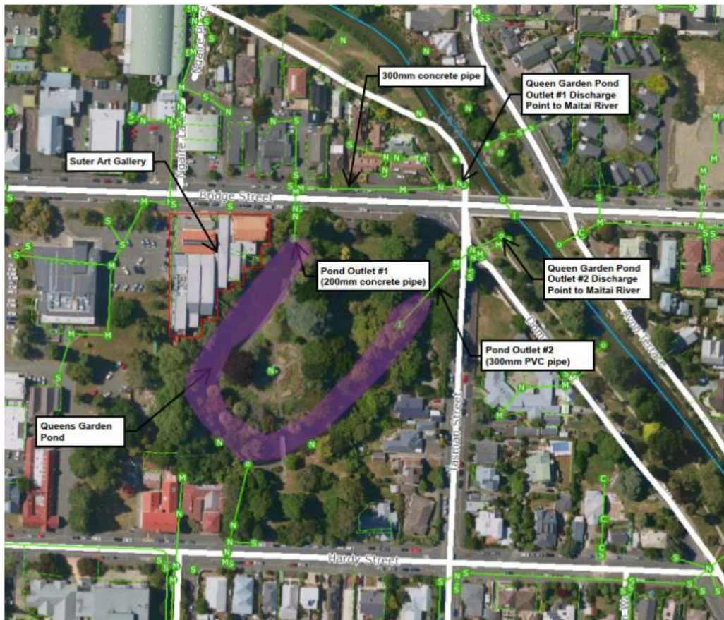
Figure 2.3: Existing drainage infrastructure site map
