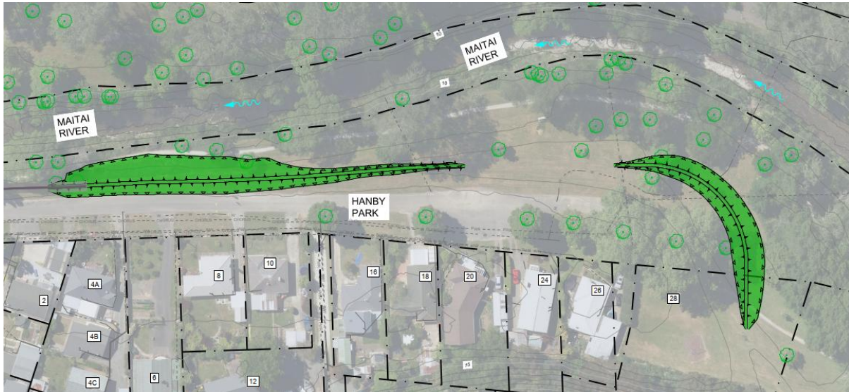
Figure 5.2: Plan showing area of stopbank raising in Portion 1, green shading.
