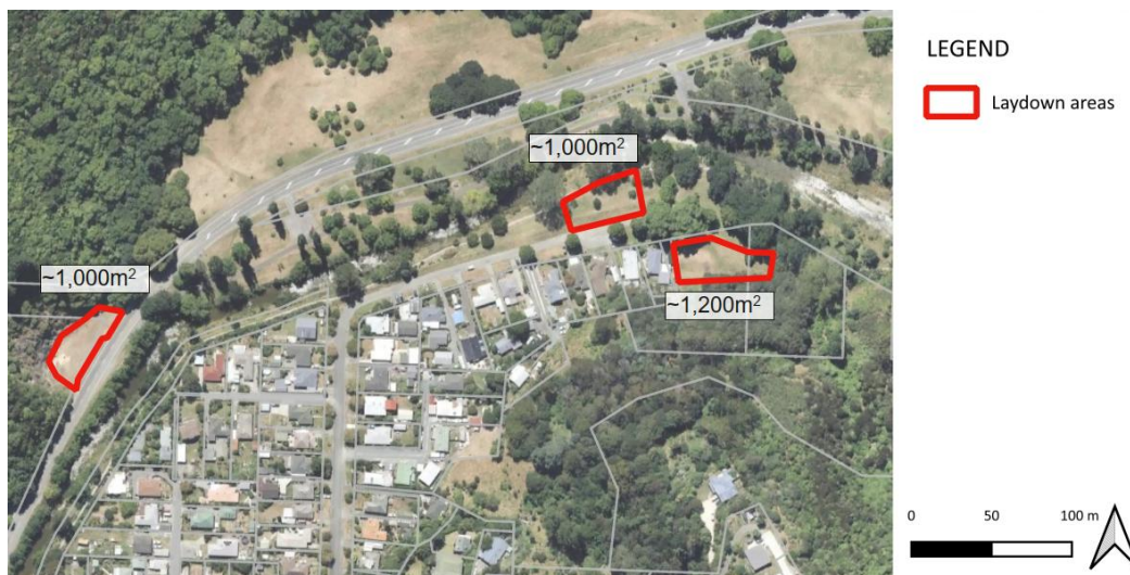
Figure 3.4: Likely construction laydown areas, shown in red
